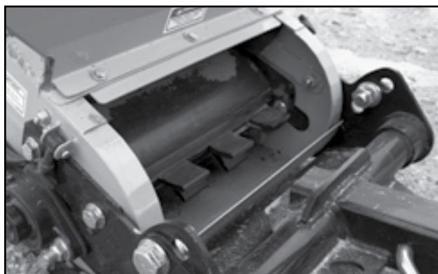
Fig 40 - Hopper end belt, guard removed
