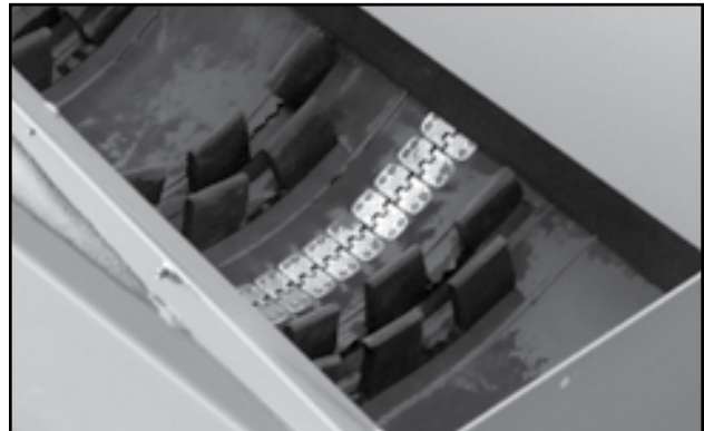
Fig 42 - Conveyor Belt Seam, as Seen in Hopper
