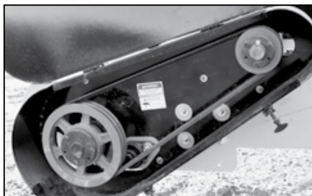
Fig 45 - Speed Reduction Drive with Guard Opened
