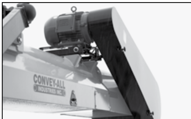
Fig 6 - Electric motor with direct drive
