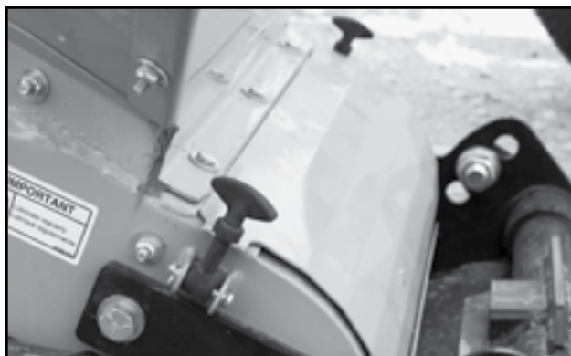
Fig 39 - Hopper end belt, guard in place
