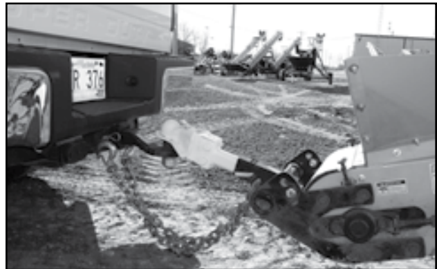
Fig 28 - Ball hitch with safety chains
