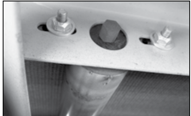
Fig 27 - Rollers are adjustable
