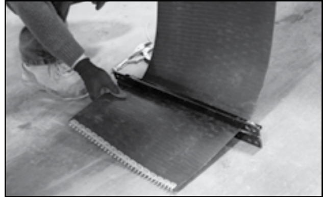
Fig 19 - Clamp the belt
