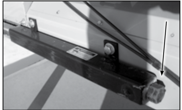
Fig 45 - Conveyor belt tensioning jacks
