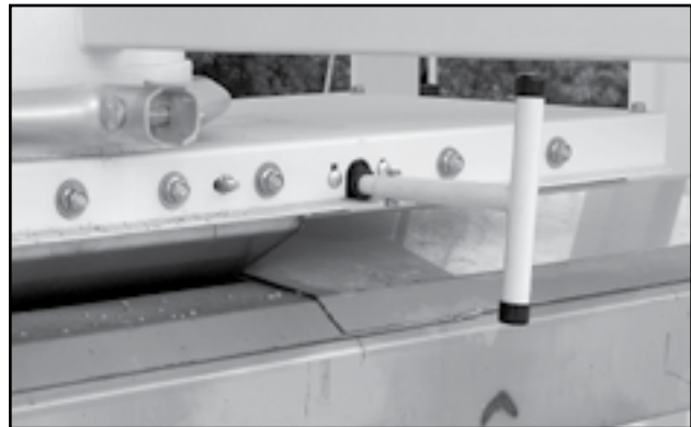
Fig 7 - Gate assembly with manual crank
