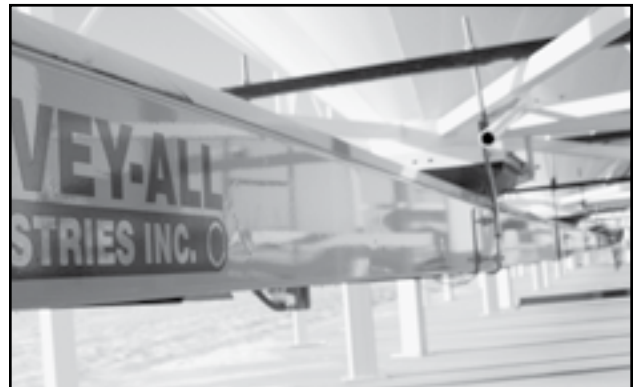
Fig 13 - Hanging bed section
