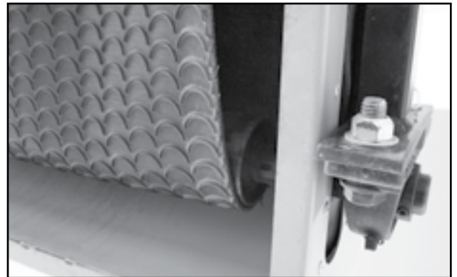
Fig 39 - Tail roller from underneath
