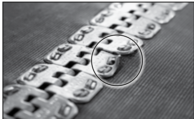
Fig 26 - Something catching on belt lacing
