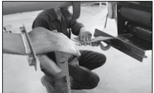
Fig 20 - Use a Come-Along Winch to pull
