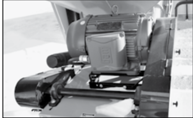
Fig 31 - Electric engine and drive assembly
