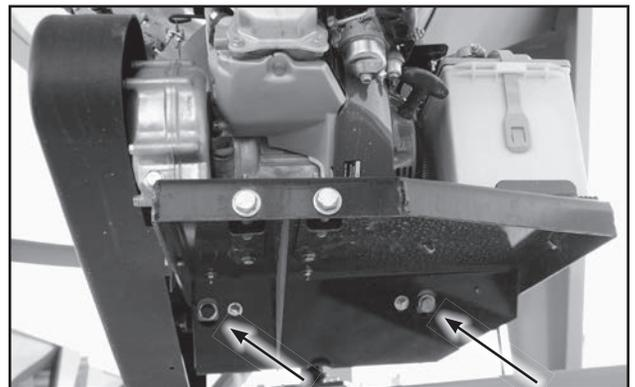
Fig 56 - Conveyor Tension Bolts
