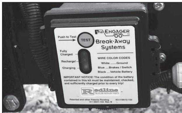
Fig 32 - Breakaway Switch Control Box
