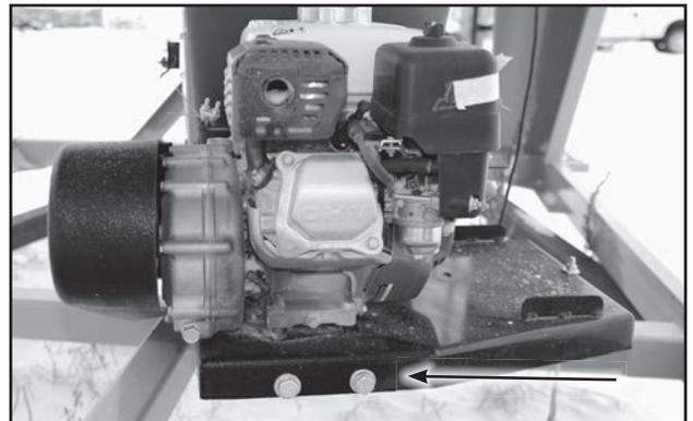
Fig 74 - Engine Mount Positioning Bolts
