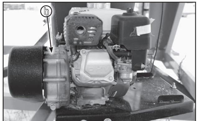
Fig 7 - Centrifugal Clutch
