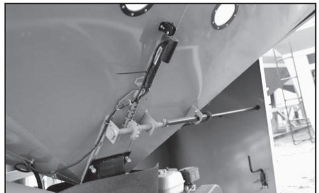
Fig 19 - Hopper Gate with Electric Actuator
