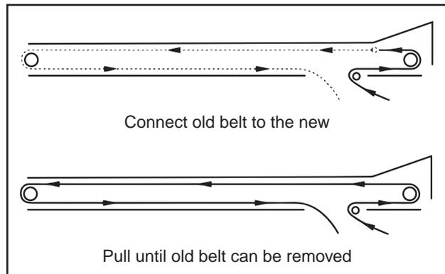
Fig 71 - Threading the Belt
