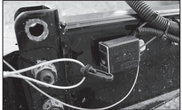
Fig 33 - Break-Away Switch with Pin Removed
