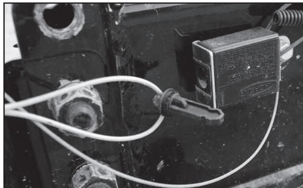
Fig 60 - Break-Away Switch Pin
