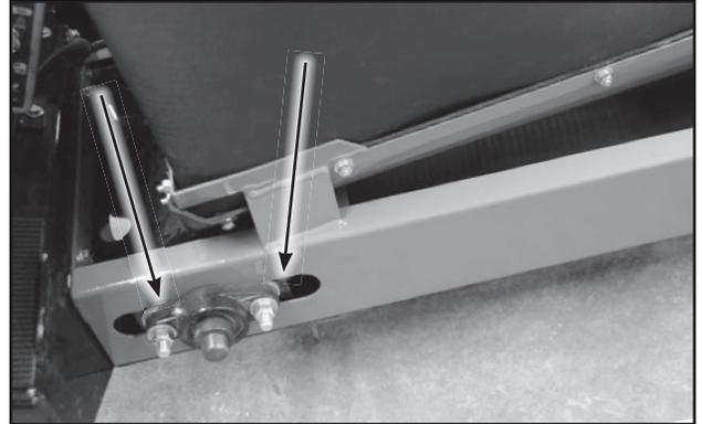
Fig 67 - Roller Bearing Anchor Bolts, Guard Removed
