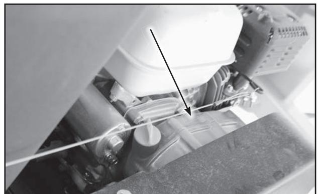
Fig 64 - Centrifugal Clutch
