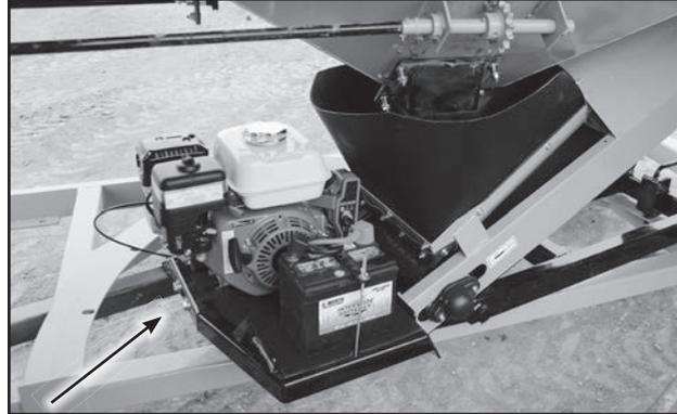
Fig 8 - Engine Mount Bolts
