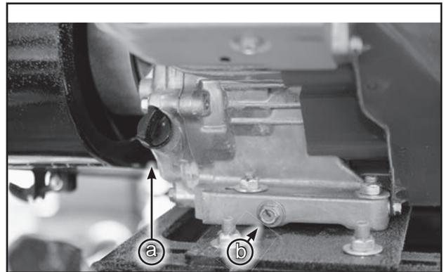
Fig 78 - Engine Oil, Fill Plug (a) and Drain Plug (b)
