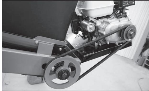
Fig 57 - Drive Belt, Guard Removed
