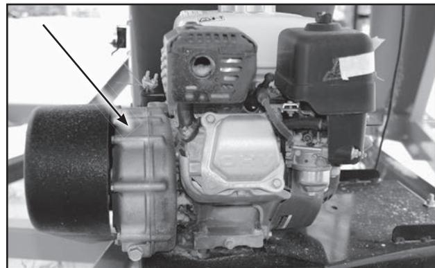
Fig 52 - Centrifugal Clutch
