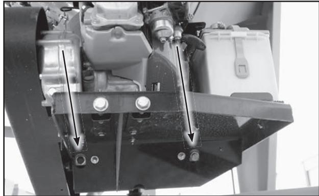
Fig 66 - Tension Bolts, Below Engine
