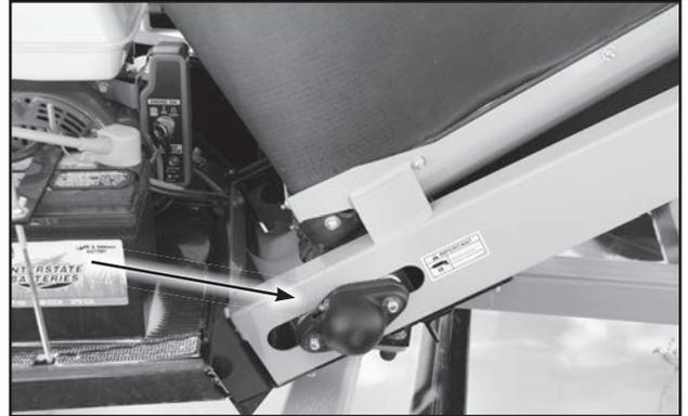
Fig 53 - Hopper Roller Bearing
