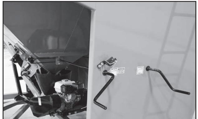
Fig 18 - Hopper Gate with Manual Levers
