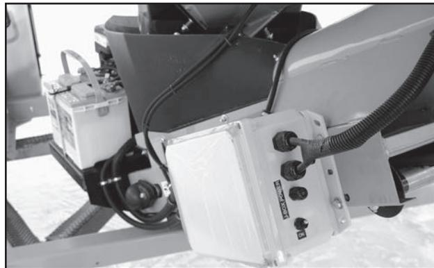
Fig 23 - Weigh Scale Receiving Box
