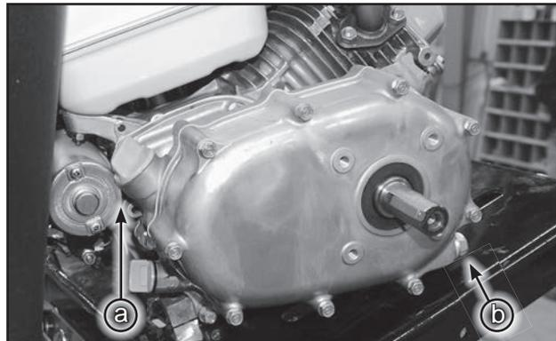
Fig 80 - Centrifugal Clutch, Fill Plug (a) and Drain Plug (b)
