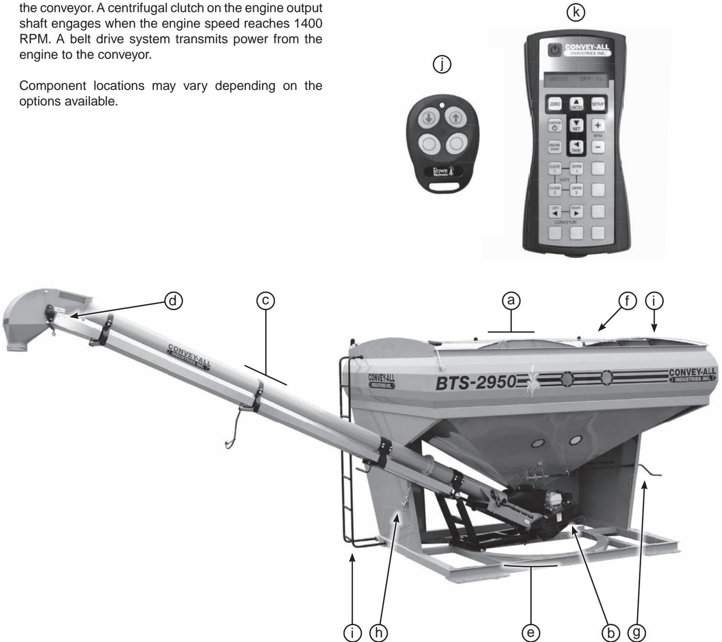
Fig 5 - BTS-2950 and Remote Control Handsets
