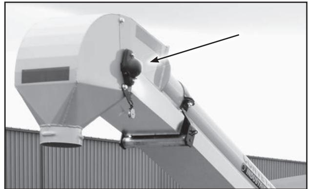
Fig 54 - Discharge Roller Bearing
