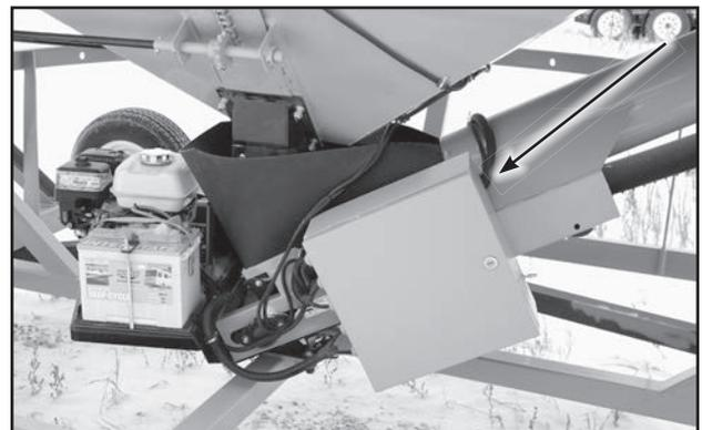
Fig 12 - Remote Control Receiver
