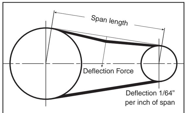
Fig 75 - Tension Calculation
