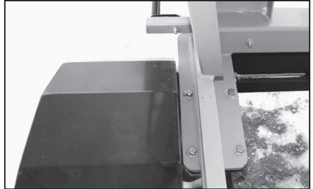
Fig 36 - Trailer Anchor Bolts
