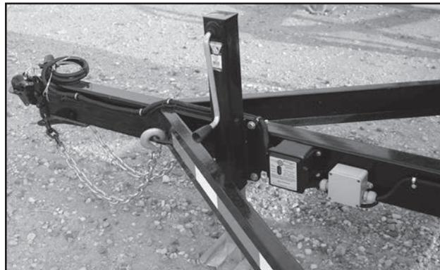
Fig 31 - Hitch, Jack, Breakaway System and Electrical Box
