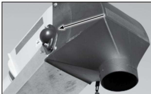
Fig 50 - Discharge roller bearing
