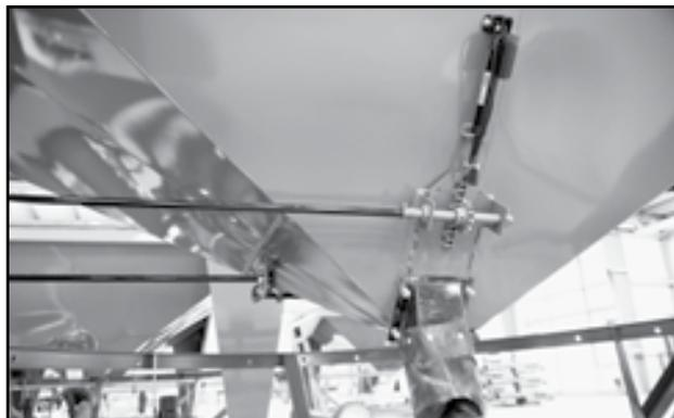
Fig 12 - Compartment gate with electric actuator
