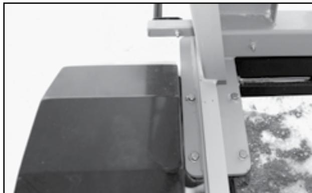
Fig 30 - Trailer anchor bolts
