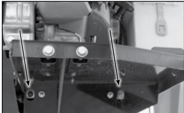
Fig 65 - Tension bolts, below engine
