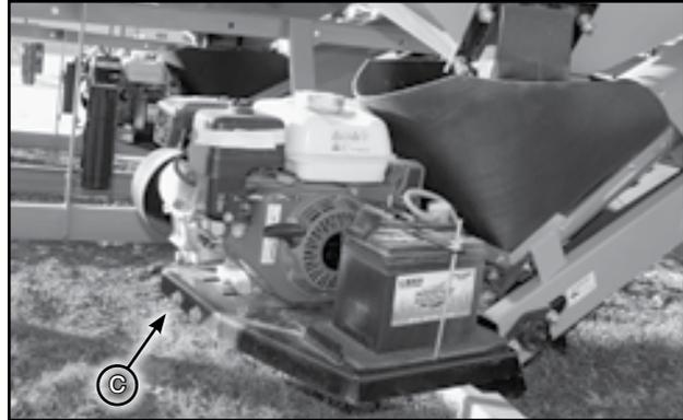
Fig 8 - Engine mount bolts
