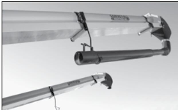
Fig 19 - Discharge spout with extension
