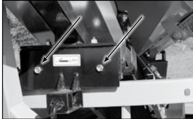
Fig 51 - Pivot roller bearings
