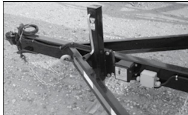
Fig 25 - Hitch, jack, breakaway system and electrical box
