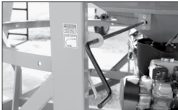
Fig 13 - Compartment gate with manual lever
