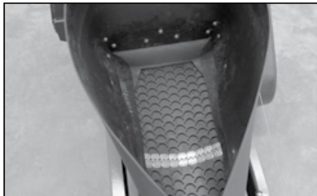
Fig 54 - Conveyor hopper, not attached to tender
