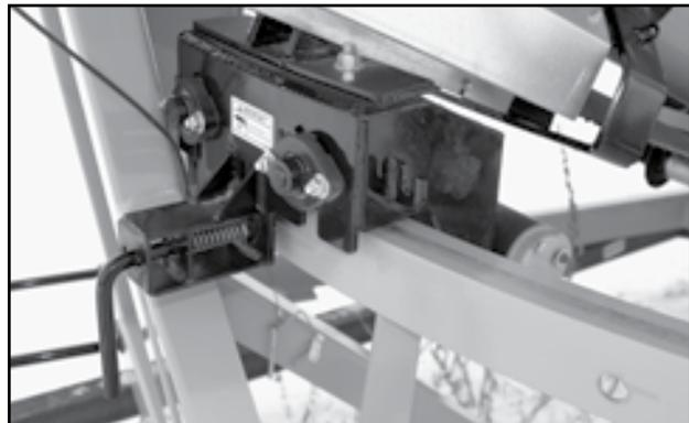
Fig 36 - Pivot roller bracket
