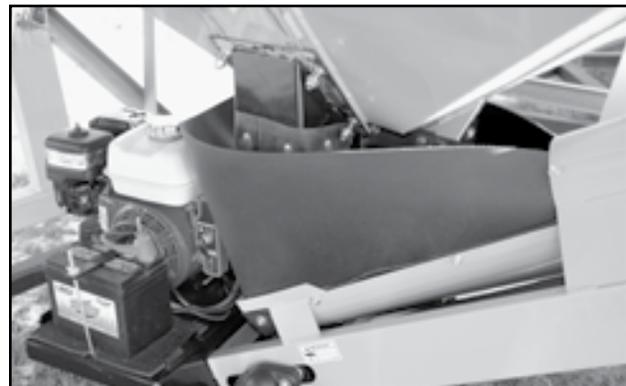
Fig 43 - Hopper gate and conveyor
