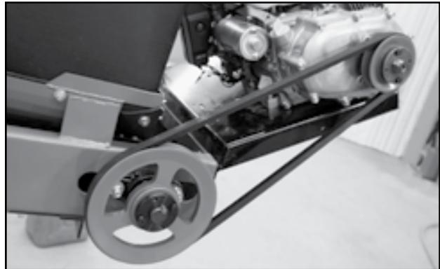
Fig 71 - Drive belt, guard removed
