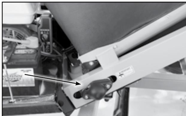
Fig 49 - Hopper roller bearing
