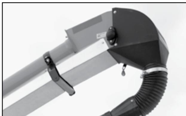
Fig 32 - Downspout fastened to discharge
