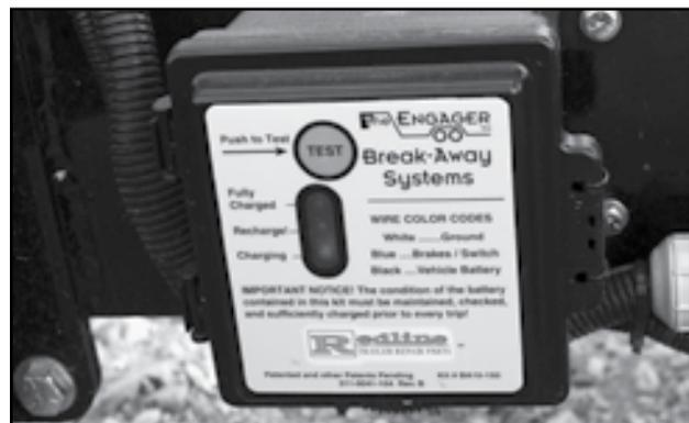
Fig 26 - Breakaway switch control box
