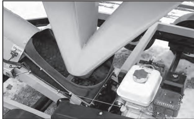
Fig 32 - Hopper Funnels and Conveyor
