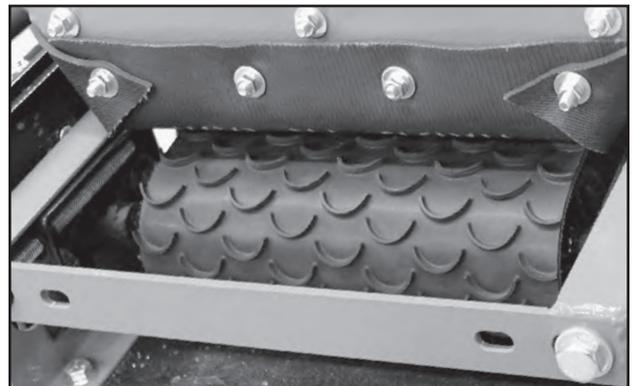
Fig 48 - Belt Aligned, Engine Removed
