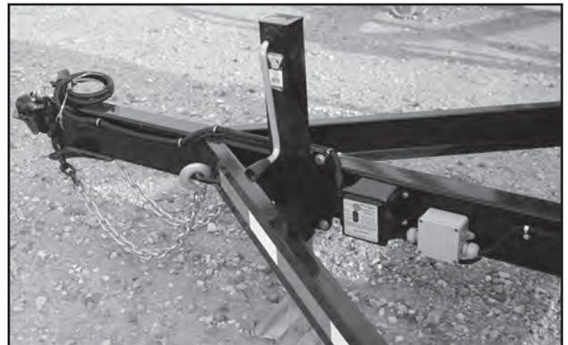
Fig 15 - Hitch, Jack, Breakaway System, Electrical Box
