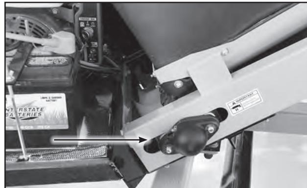
Fig 36 - Drive Roller Bearings
