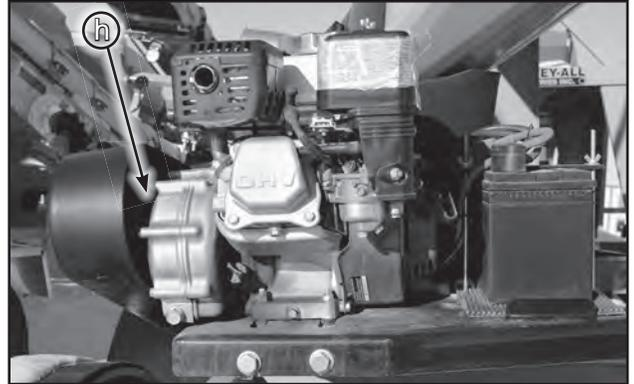
Fig 6 - Centrifugal Clutch
