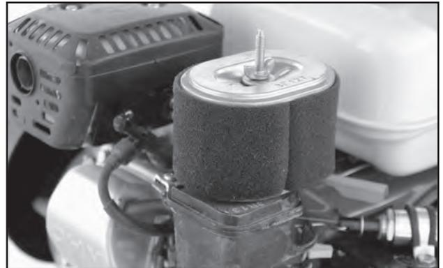
Fig 58 - Air Filter with Cover Removed
