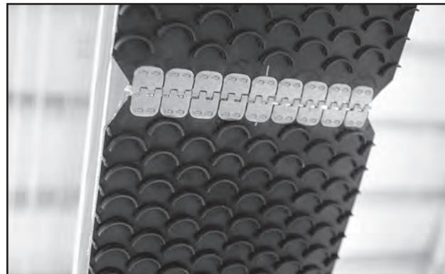
Fig 50 - Conveyor Belt Beneath Wind Guard
