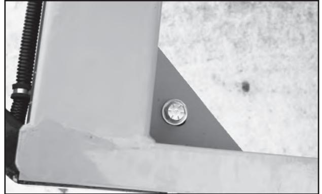
Fig 20 - Trailer Anchor Bolts
