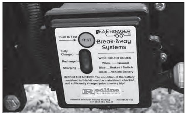
Fig 16 - Breakaway Switch Control Box
