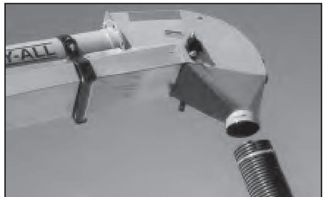
Fig 22 - Slide Down Spout Over Discharge Spout
