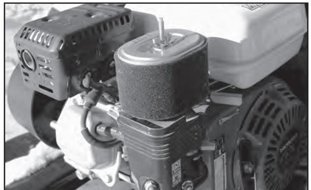
Fig 41 - Air Filter, Cover Removed
