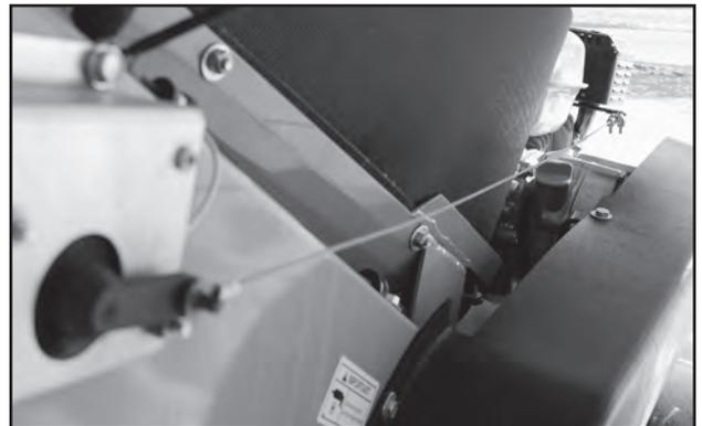
Fig 30 - Remote to Throttle Cable
