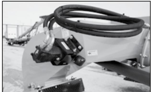
Fig 42 - Hydraulic Motor
