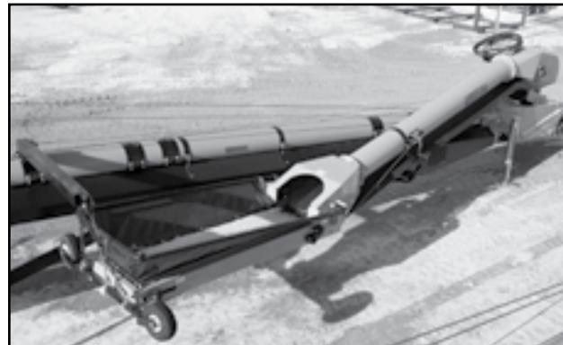
Fig 23 - Swing-Out Conveyor
