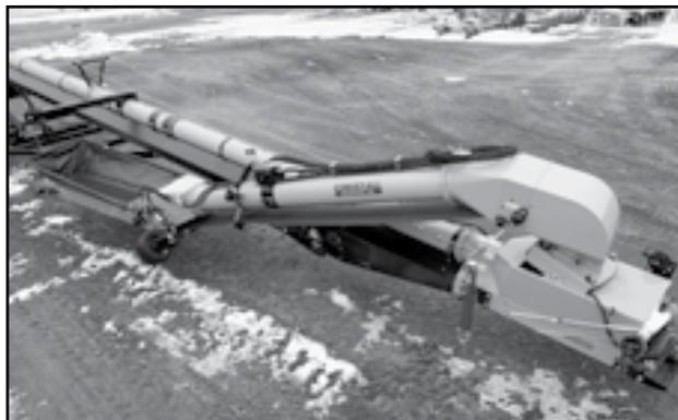
Fig 32 - 10 Inch Hydraulic Drive Swing Out (Optional)
