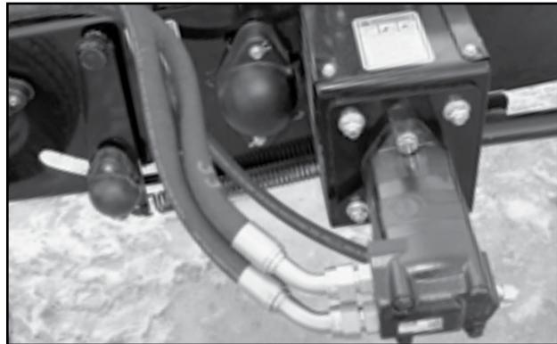
Fig 95 - Hydraulic Drive, Main Conveyor
