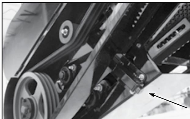
Fig 92 - Drive Belt Tension Bolt
