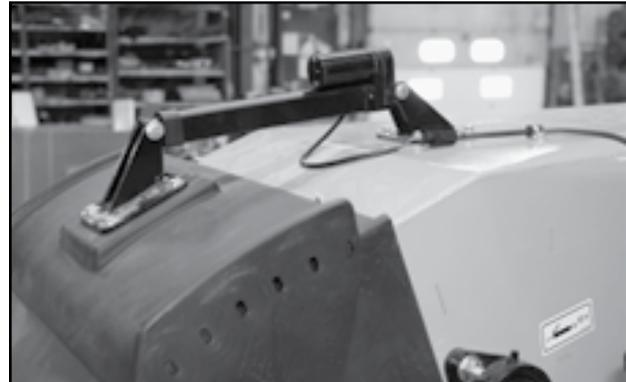
Fig 22 - Discharge Spout with Electric Actuator
