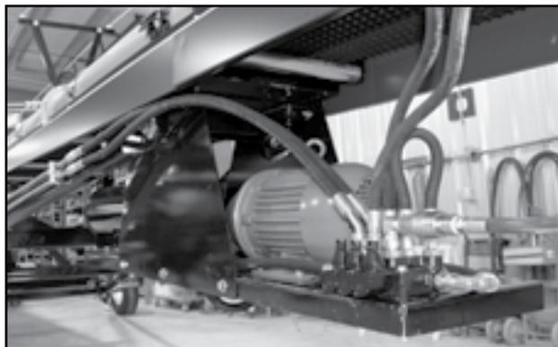
Fig 11 - Electric Motor to Hydraulics
