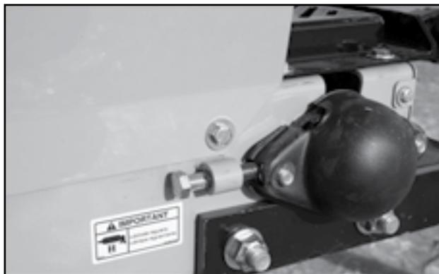
Fig 83 - Hopper Roller Bearings
