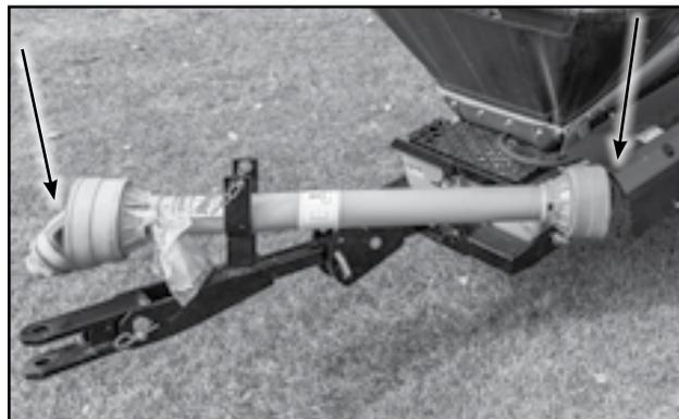
Fig 80 - Grease End PTO
