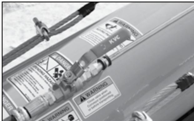
Fig 17 - Hydraulic Valve to Conveyor Tube Cylinders
