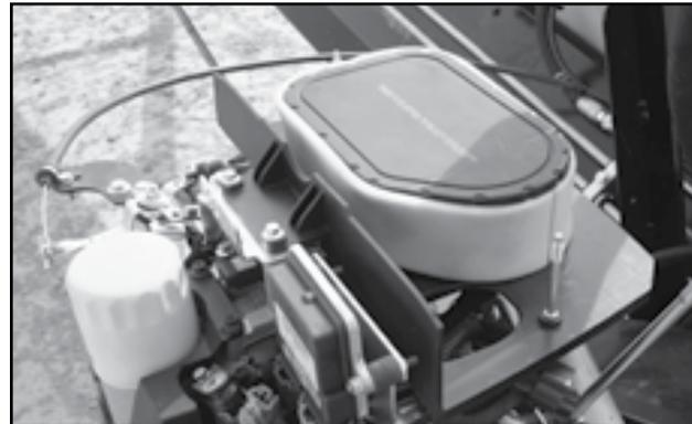
Fig 122 - Air Filter, Cover Removed
