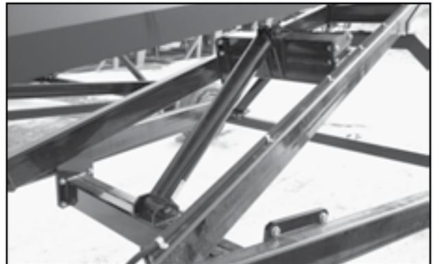
Fig 99 - Tube Lift Cylinder
