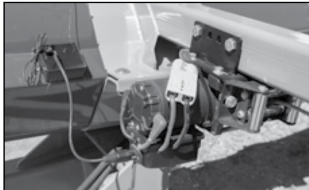
Fig 45 - Electric Winch
