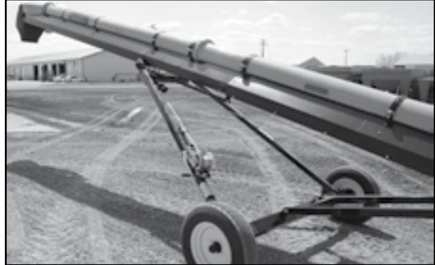
Fig 28 - A-Frame Undercarriage
