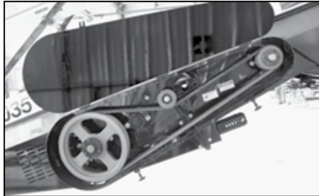
Fig 114 - Counter Shaft to Drive Belt with Guard Open
