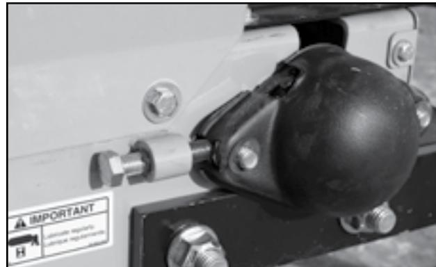
Fig 106 - Adjustment Bolts on Hopper without Transition
