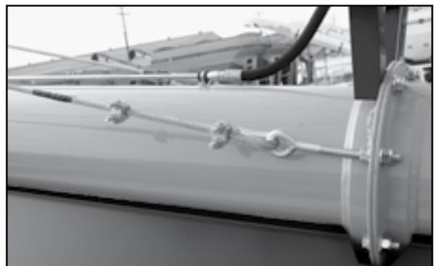
Fig 100 - Cable Bridging Eye Bolts
