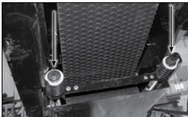
Fig 90 - Tension Bolts, Spring Tension Drive Box
