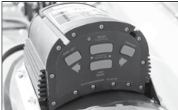
Fig 47 - Electric Controller for Mover Kit
