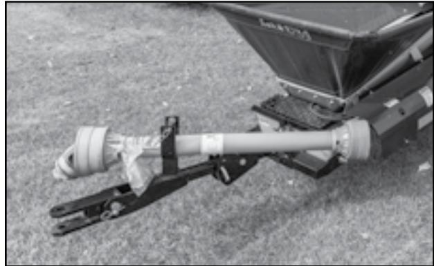
Fig 73 - PTO Stored on Hitch
