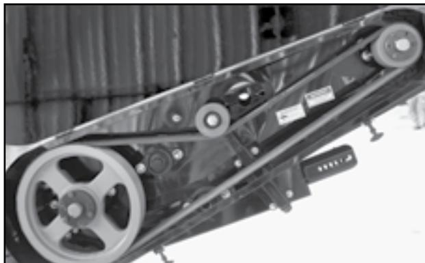
Fig 117 - In-Line Drive with Guard Opened
