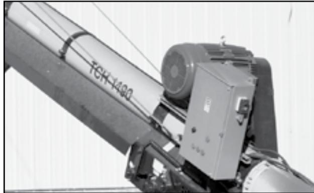
Fig 59 - Motor Control Box
