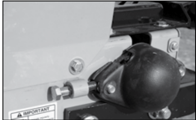
Fig 52 - Adjustment bolts on hopper
