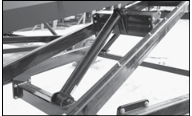
Fig 63 - Steering wheel lift cylinder
