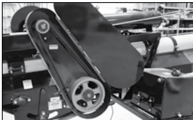
Fig 81 - Belt drive with guard opened
