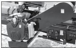
Fig 64 - Gas Engine
