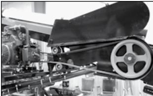
Fig 115 - Engine to Counter Shaft with Guard Open
