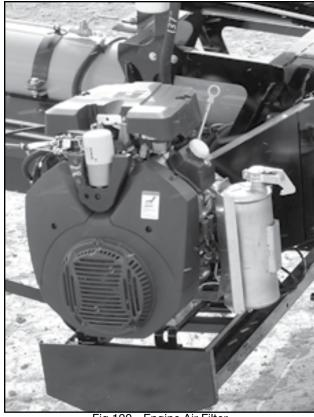
Fig 120 - Engine Air Filter
