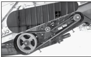
Fig 114 - Counter Shaft to Drive Belt with Guard Open
