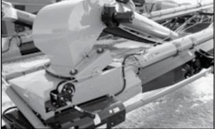
Fig 36 - Swing-out Discharge to Main Conveyor Hopper
