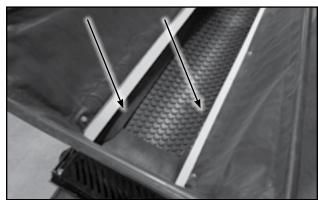
Fig 94 - Hopper Flashing
