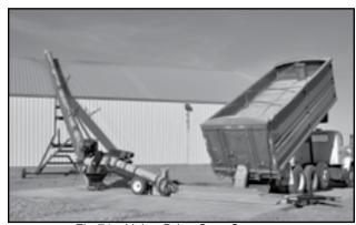
Fig 71 - Using Drive Over Conveyor
