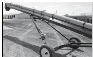
Fig 28 - A-Frame Undercarriage
