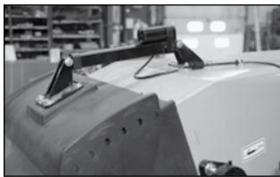
Fig 22 - Discharge Spout with Electric Actuator
