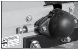
Fig 106 - Adjustment Bolts on Hopper without Transition
