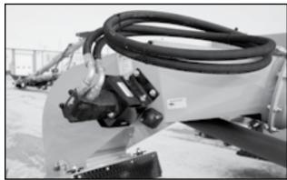
Fig 42 - Hydraulic Motor
