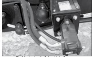
Fig 95 - Hydraulic Drive, Main Conveyor
