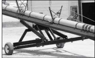
Fig 29 - Scissor Lift Undercarriage
