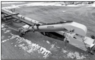
Fig 32 - 10 Inch Hydraulic Drive Swing Out (Optional)
