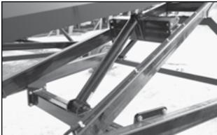
Fig 99 - Tube Lift Cylinder
