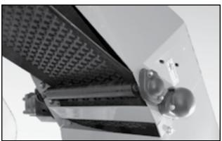
Fig 86 - Discharge Rollers on Swing Out
