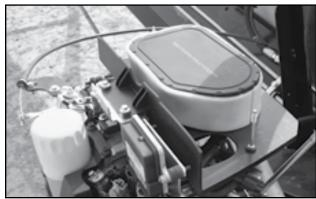
Fig 122 - Air Filter, Cover Removed
