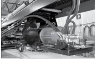
Fig 11 - Electric Motor to Hydraulics
