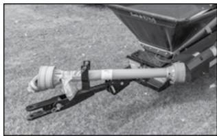
Fig 73 - PTO Stored on Hitch
