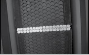
Fig 109 - Conveyor Belt Seam, as Seen in Hopper
