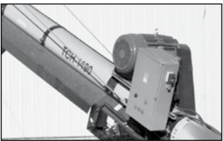
Fig 59 - Motor Control Box
