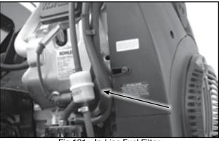
Fig 121 - In-Line Fuel Filter
